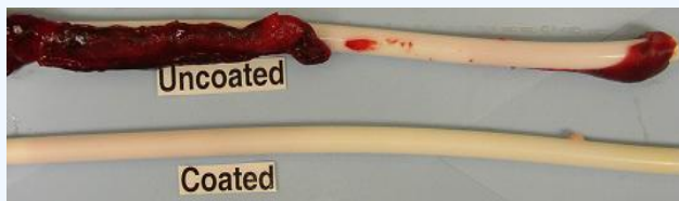
Uncoated and coated samples explanted after 30 days.
