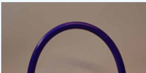
Poly(urethane) catheter coated with Astute® and subjected to the 'wet glove' test. Toluidine blue dye indicates a homogenous coating that has remained intact.
