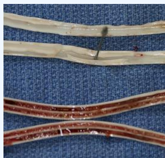
Internal surfaces of coated (top) and uncoated (bottom) samples used during blood loop study.
